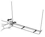
2. Container for the drained water: Place a low and wide container under the water filter in order to collect the residual water.
