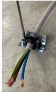
Fix power cord to the plastic holder.
