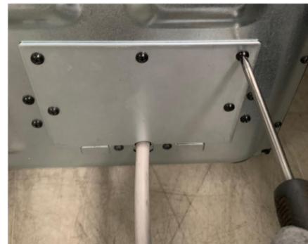
Assemble cover and tighten screws.
