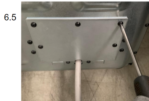
Assemble cover and tighten screws.
